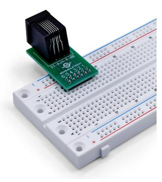
The breakout board can be connected as shown on the left to minimize the amount of breadboard space required.
